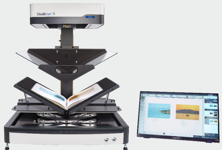
Scanning highly glossy originals with V-shaped glass plate.
